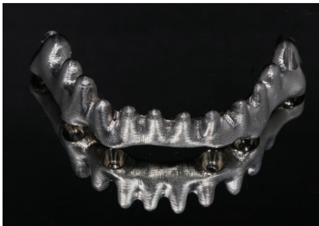
Figure 13. Lower framework milled in titanium.
