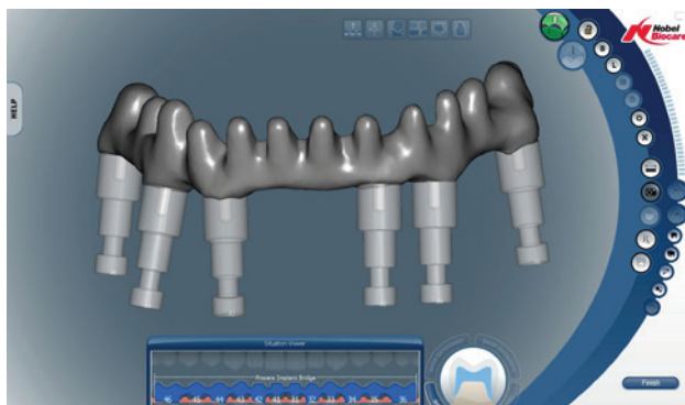
Figures 10 and 11. Using the NobelProcera CAD/CAM software, shape, midlines, shade, gingival margin position and cleansibility are carefully managed.
